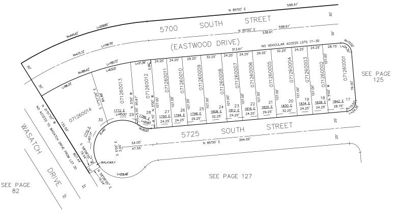
5' UTILITY & DRAINAGE EASEMENTS EACH SIDE OF PROPERTY LINES AS INDICATED BY DASHED LINES, EXCEPT AS OTHERWISE SHOWN.
